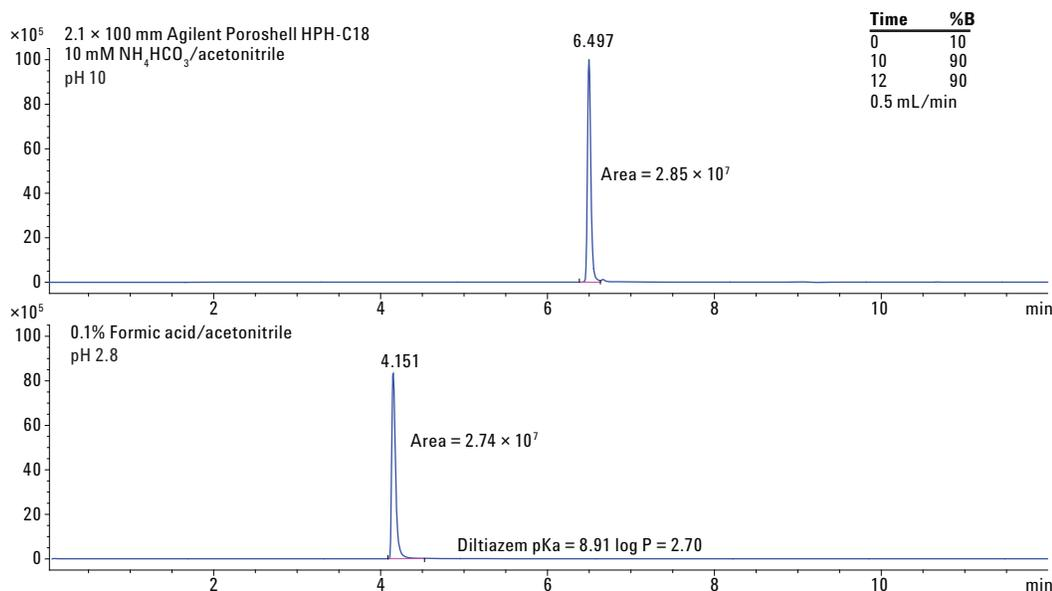
Figure 4C. Comparison of LC/MS of bases (diltiazem, pKa 8.91, logP 2.70) in positive ion electrospray mode at high and low pH. Agilent Poroshell HPH-C18, 2.1 × 100 mm.
