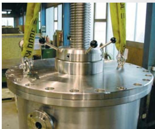
600 mm i.d. column as a special reactor for coating processes. Integrated level indicators assist assembly / disassembly for maintenance purposes.
