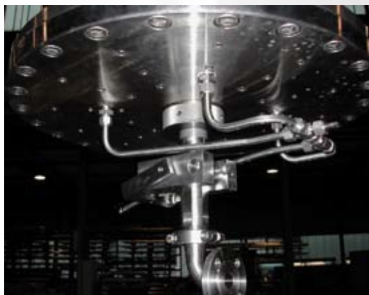
600 mm i.d. column, slurry outlet with separate tap, quadruple eluent outlet.
