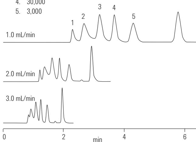
**Figure 6.** Take care to choose the best flow rate, depending on the particle size of the column.
