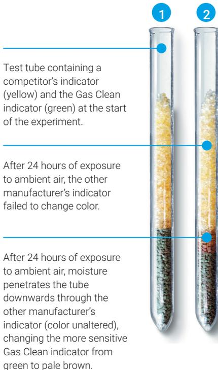
Test tube containing a competitor's indicator (yellow) and the Gas Clean indicator (green) at the start of the experiment.
