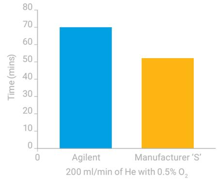
**Figure 8.** When using gas clean filters to clean He containing 0.5% O<sub>2</sub> flowing at 200 mL/min, the Agilent Gas Clean Filter changed color at 70 mins while the manufacturer 'S' filter changed color at 52 mins.
