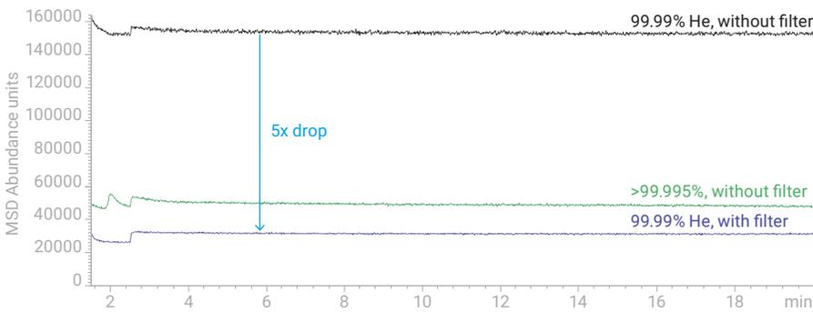
**Figure 6.** EICs (32 *m/z*) for O<sub>2</sub>: A comparison of balloon grade (99.99%) He (with and without a carrier Gas Clean Filter) and higher grade (>99.995%) He (without filter). Using a carrier gas filter with balloon grade He dropped the O<sub>2</sub> abundance to levels lower than the higher grade He (>99.995%) without a filter.
