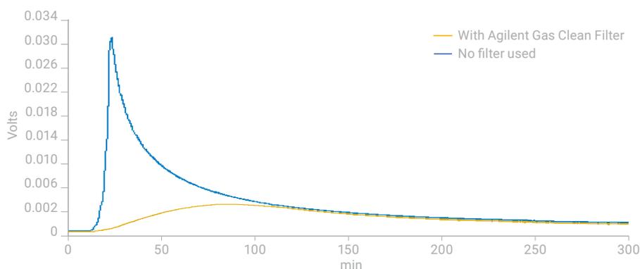
**Figure 2.** The difference in bleed levels of two GC columns due to moisture exposure, with and without a filter, when running a temperature program (50 °C to 350 °C at 20 °C/min). When no filter is used, an extreme rise in the bleed profile is clearly visible due to moisture in the carrier gas. By using Gas Clean Filters, a normal bleed profile is achieved with the removal of all moisture in the carrier gas.
