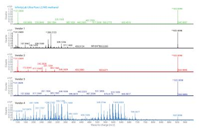
Figure 1. Full scan direct infusion comparison of four vendors and Agilent InfinityLab Ultra-Pure LC/MS methanol in positive polarity using an Agilent 6550 iFunnel Q-TOF LC/MS *m/z*. 121 and 922 are reference solution ions.
