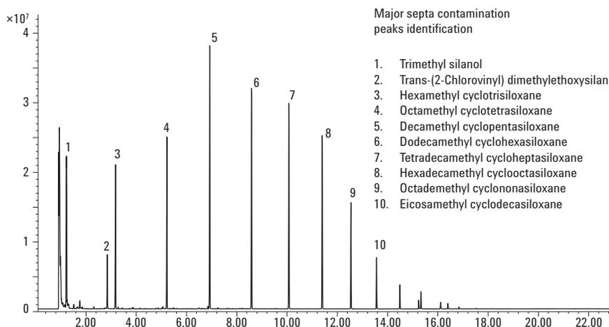
Figure 1. GC/MS HS chromatogram of vial blank with PTFE/silicone headspace septum heated to 300 °C shows that the PTFE/silicone septum causes significant contamination when heated at high temperature.
