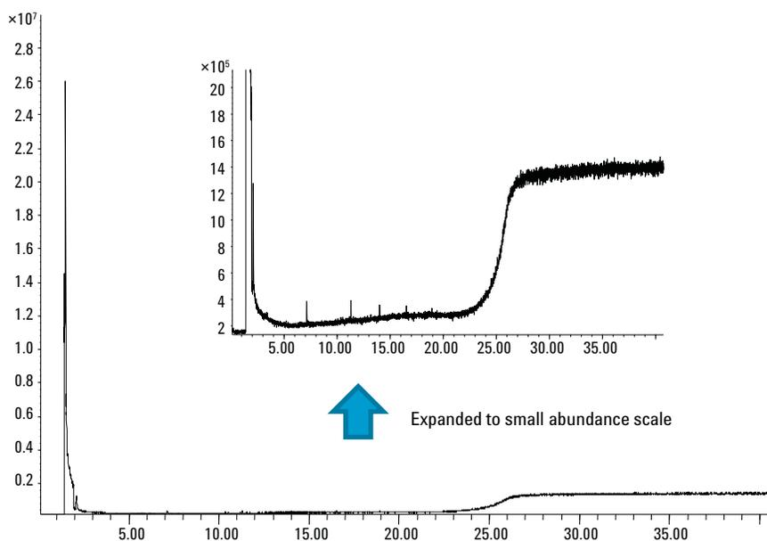
Figure 5. GC/MS chromatogram of HS background with High Performance septum. Vials were equilibrated at 300 °C for 30 min and data were acquired with MS scan range of 35-550 amu.
