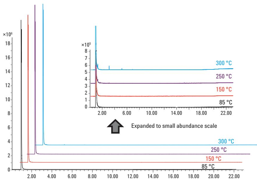
Figure 3. GC/MS chromatogram comparison of vial blanks with High Performance septa at different temperatures. Vial blanks were equilibrated at each temperature for 30 min and initially pressurized to 15 psi but then vented to 10 psi prior to injection.
