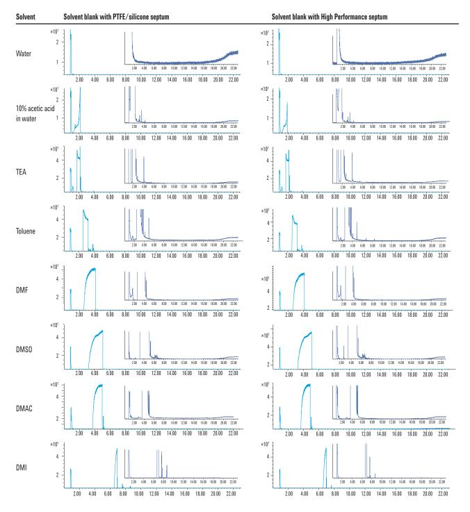
Figure 6. GC/MS HS chromatograms of solvent blanks with PTFE/silicone septum and High Performance septum. The High Performance septum results do not indicate any incompatibilities with common headspace solvents.
