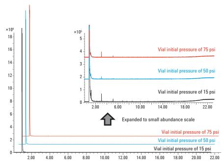
Figure 4. GC/MS chromatogram comparison of vial blanks with High Performance septa at different pressures. The pressure represents the initial pressure each vial was charged to prior to venting. All vials were vented to 10 psi before injection. Vials were equilibrated at 300 °C for 30 min.
