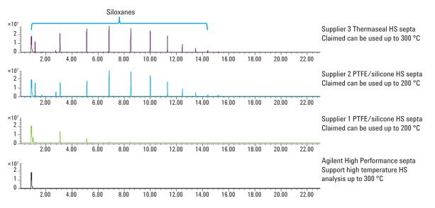
Figure 2. GC/MS chromatographic comparison of vial blank with different PTFE/silicone headspace septa and High Performance septum. Vials were equilibrated at 300 °C for 30 min. By using High Performance septa, the vial blank chromatogram clearly shows a significantly cleaner HS chromatographic background.
