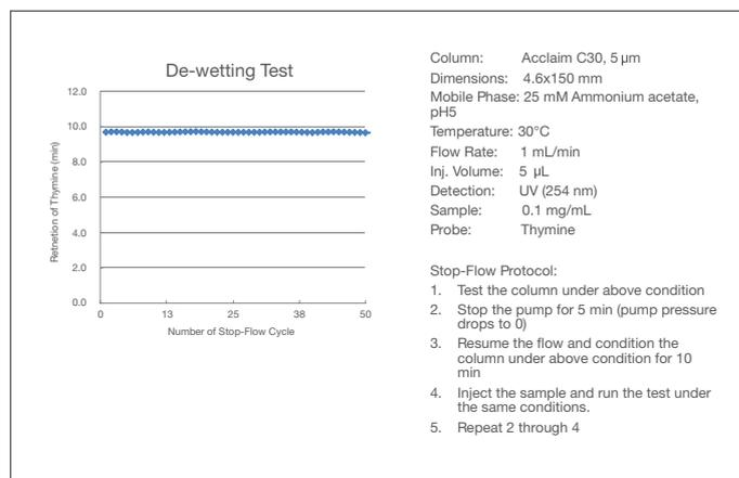
**Figure 3.** Aqueous compatibility of the Acclaim C30 column.
