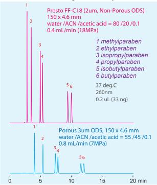
When mobile phase composition and flow rate is optimized, Presto FF-C18 can at times achieve amazing peak shape for small molecules.
