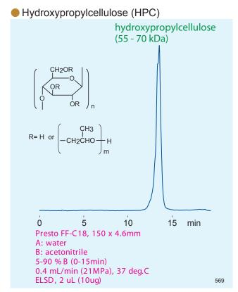
Hydrophilic polymers, which have been traditionally analyzed on aqueous SEC (GFC) mode, may now also be analyzed on Presto FF-C18 with RP mode and gradient elution.
