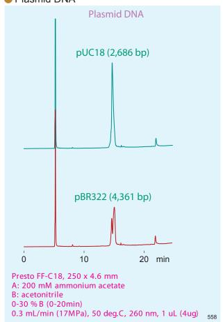
Double stranded DNA is a tremendously large molecule that is normally hydrolyzed into fragments (via nuclease) prior to analysis. Presto FF-C18 can analyze intact DNA as well as DNA fragments.
