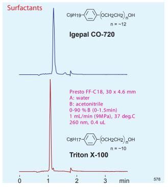
With small compounds, Presto FF-C18 sometimes shows worse separation than porous ODS columns. Igepal and Triton are mixtures of different oxyethylene chain lengths. Porous ODS column can easily separate the oligomers, while Presto FF-C18 provides poor selectivity due to low oxygen recognition. However, having the oligomers co-elute on Presto FF-C18 can be favorable since it produces one peak in a short time analysis.
