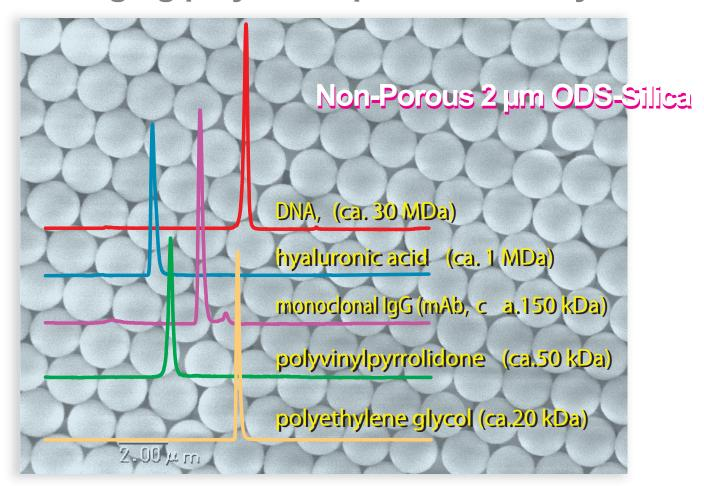
Imtakt has developed a novel 2um non-porous high resolution ODS column.
