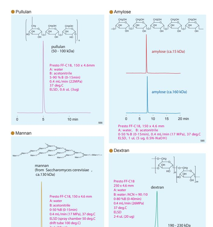
Reversed-phase separation for non-ionic polysaccharides on Presto FF-C18 does not require any pH modifier. Excellent peak shape was observed for several non-ionic polysaccharides using water / acetonitrile gradients. Polysaccharides contain multiple OH groups, and different concentrations of acetonitrile may be required for proper elution. The data shows that retention will be similar for homo polysaccharides larger than 10kDa. Peak shape is dependent upon molecular size distribution.
