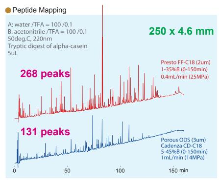
Presto FF-C18 enables unbelievable separation power for peptide mapping. Accurate trace analysis for peptides is very important for proteome analysis, but can be compromised with porous ODS column - due to adsorption in micro-pores.
