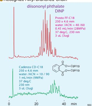
On conventional porous ODS, Phthalic di-ester has numerous branched-chains with the same MW that co-elute. In contrast, Presto FF-C18, at a low flow rate, recognizes the alkyl chain isomers and is more sensitive.
