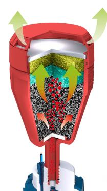
S.C.A.T. exhaust filters block off harmful vapours and ensure for safe pressure equalization in the waste containers of HPLC systems. Our core active carbon has been optimized for taking up organic solvent vapours and has been tested, using official ASTM/DIN/ISO test methods.
