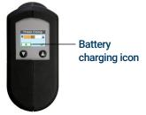
2 Charging is complete when the green battery fill scrolling stops and the icon is solid green. Disconnect the power cord from the crimper.
