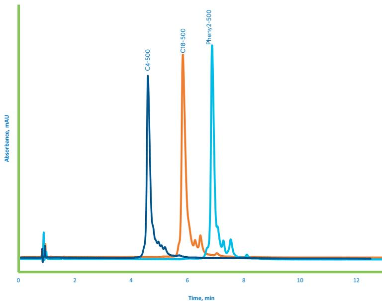
500 Å is a suitable pore size for the reversed-phase separation of antibodies of approximately 150 kDa in molecular weight. The 500 Å pore size retains the mAb well and a difference can clearly be observed when comparing the three different stationary phases. This is a useful tool to enable clear separation of the protein of interest from any similar compounds such as mAb fragments or impurities with similar retention.
