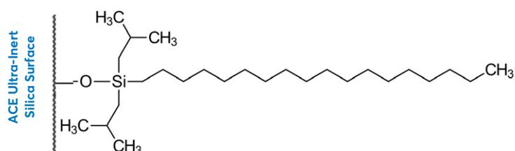
**C4:** Reversed-phase material for separations requiring a stationary phase with lower hydrophobicity. This is an important phase for large proteins given that the net interaction caused by the hydrophobic interaction is often strong in such molecules. The butyl ligand is well established in RP protein applications. This phase is well suited to the analysis of hydrophobic proteins over 5 kDa molecular weight.
