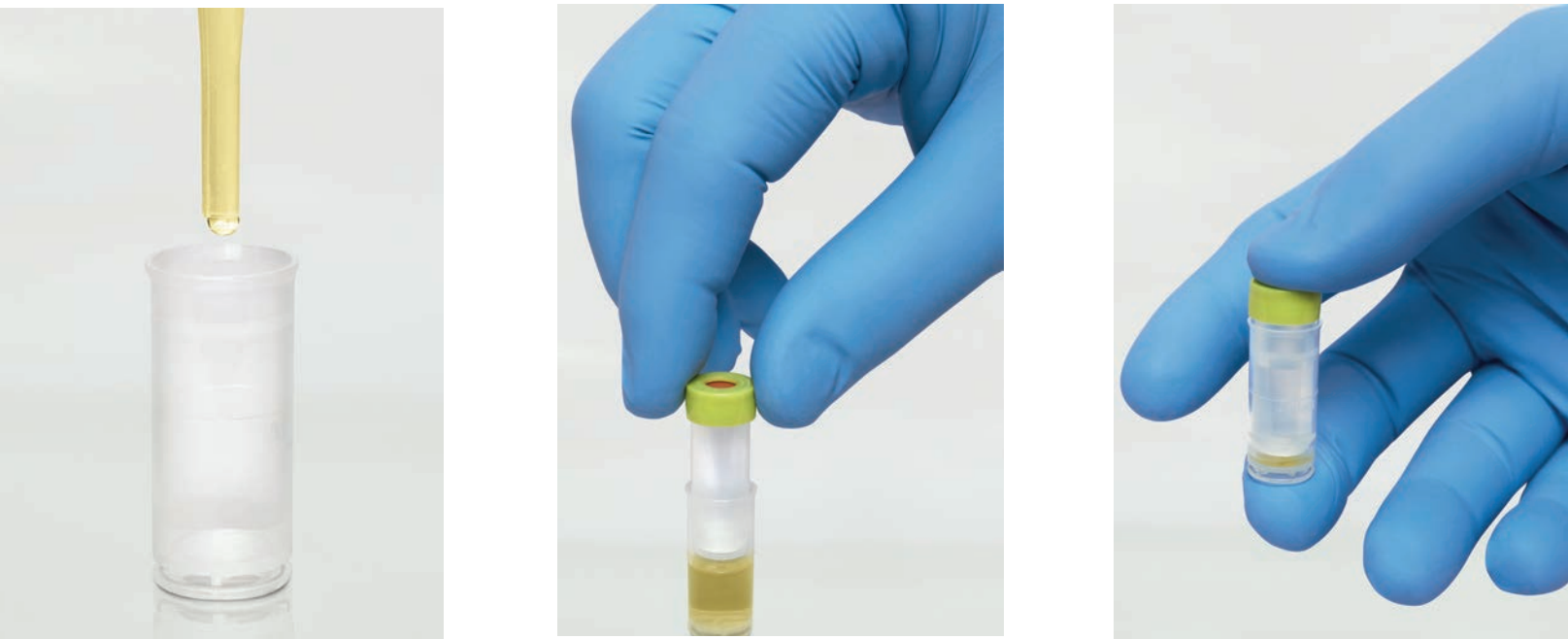
How to use Agilent Captiva filter vials
