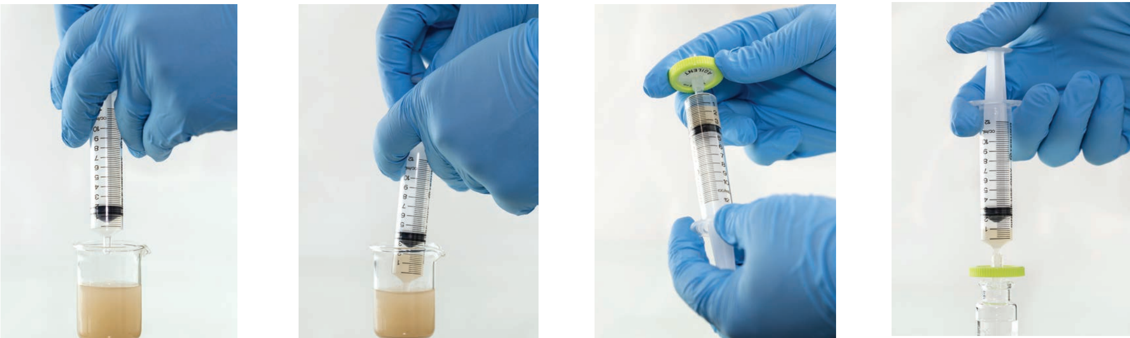
How to use Agilent Captiva syringe filters
