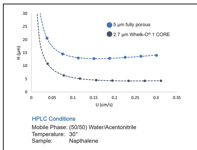
WHELK-O<sup>®</sup> 1 Core provides higher column efficiencies than similarly-sized fully porous particles, even at higher mobile phase linear velocities. H vs U curves compare performance of 2.7  $\mu\text{m}$  WHELK-O<sup>®</sup> 1 Core and 5  $\mu\text{m}$  fully porous WHELK-O<sup>®</sup> 1.
