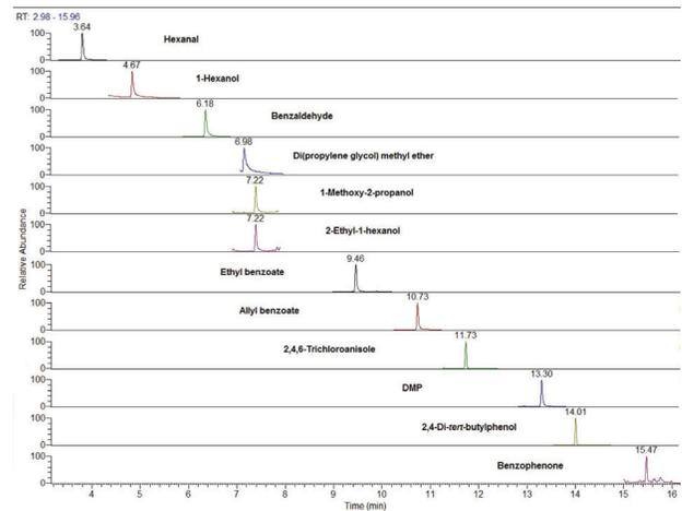
Figure 4. Chromatogram of spiked paperboard with 12 packaging migrants ( $c = 0.024\text{--}30\text{ mg/kg}$ )
