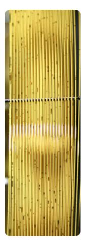
After passing the visual examination, columns are tested against the tightest QC performance specifications in the industry for efficiency, retention, selectivity and bleed. Figure shows a recently purchased competitor's PLOT column. Although it passed the competitor's QC testing, this column would have never passed the Agilent inspection and would never have been shipped to our customers.
