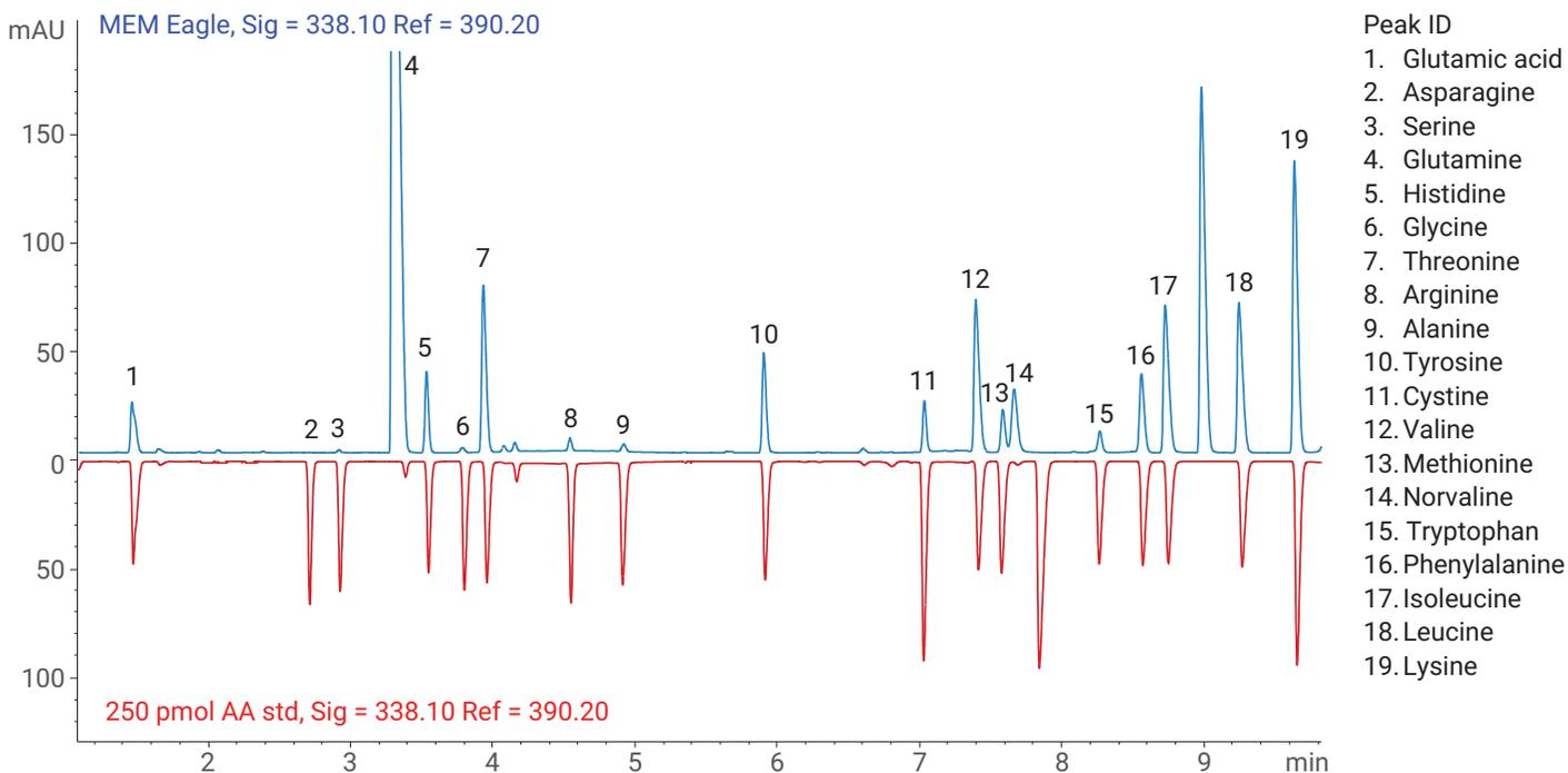
**Figure 2.** Example separation of OPA and FMOC labeled amino acids using the AdvanceBio Amino Acid Analysis column.<sup>5</sup>
