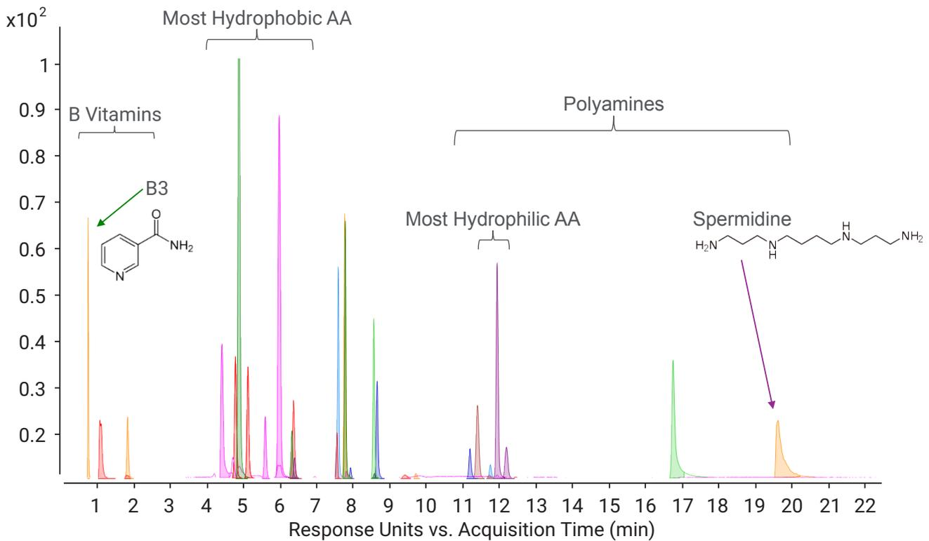
**Figure 3.** Sample separation of amino acids, B vitamins, and polyamines using the AdvanceBio MS Spent Media column with TOF detection.<sup>8</sup>
