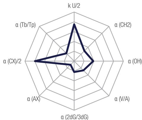
**This bare silica material offers good hydrophobic and hydrophilic selectivity.** Good absolute retention and some isomeric selectivity are demonstrated. Very strong cation-exchange properties exhibited by this acidic phase.
