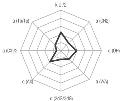
The tertiary amine functionality from the polyethyleneimine bonding of this phase shows anion-exchange activity with good hydrophilic selectivity
