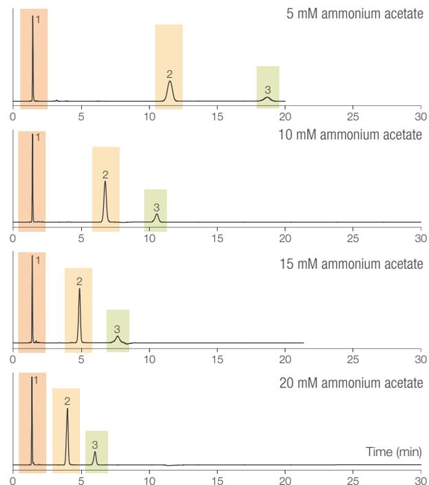
From the chromatograms above it is also evident that the increased salt concentration is beneficial to the peak shape, with sharper peaks when 20 mM ammonium acetate is used.
