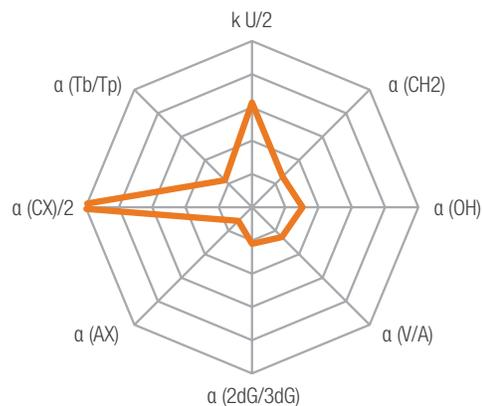
**This bare silica material offers good absolute retention, good hydrophobic and hydrophilic selectivity and some isomeric selectivity.** Very strong cation-exchange properties are demonstrated by this acidic phase.
