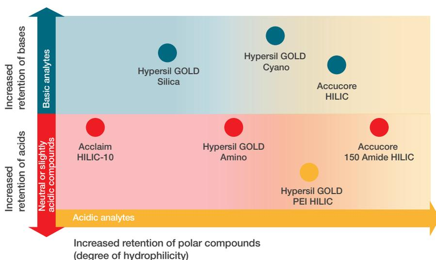
**Figure 4. Relative polarity and ion-exchange characteristics for various HILIC phases (based on study illustrated in next section)**
