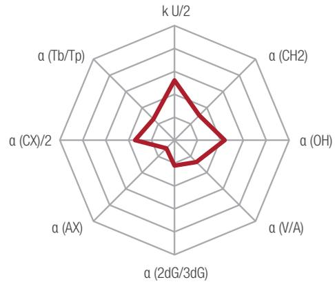
This material offers good hydrophobic, hydrophilic and isomeric selectivity and some cation-exchange properties
