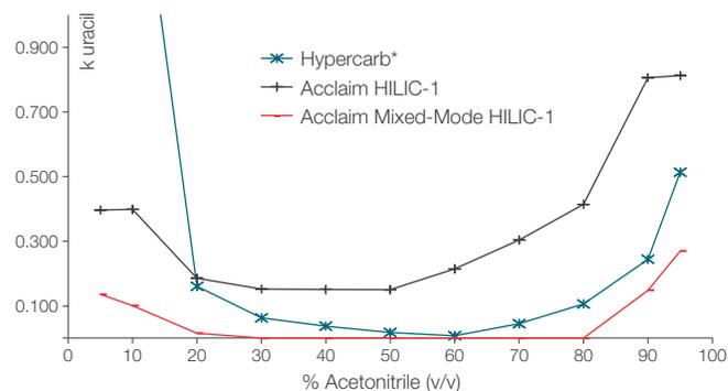
\*Although Hypercarb is not a polar stationary phase, it was included in this study because of its dual behavior (RP and HILIC), depending on the percentage of organic in the mobile phase, which allows its use for the retention of polars in RP and HILIC.
