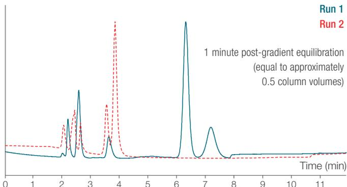
**Accucore 150-Amide-HILIC column, 2.6  $\mu$ m, 100  $\times$  2.1 mm**
