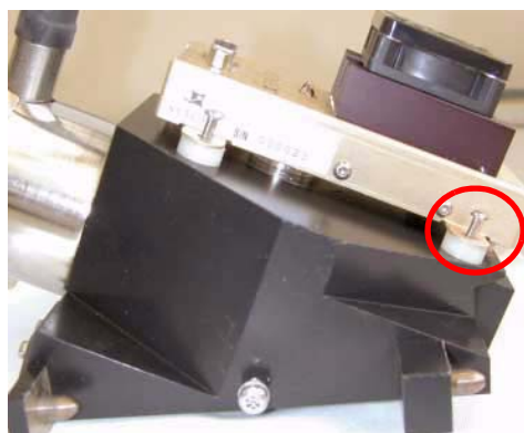
Figure 36 UV lamp should extend 6 mm (left). Lamp drive module should lie flat (right). Make sure switch is located on contact pin (circled above).
