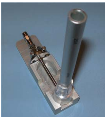
Figure 6 Electrospray nebulizer needle in needle holder
