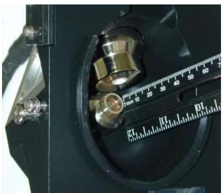
Figure 36 UV lamp should extend 6 mm (left). Lamp drive module should lie flat (right). Make sure switch is located on contact pin (circled above).
