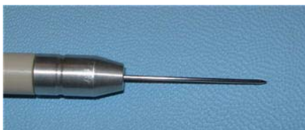
Figure 30 APCI corona needle after cleaning.
