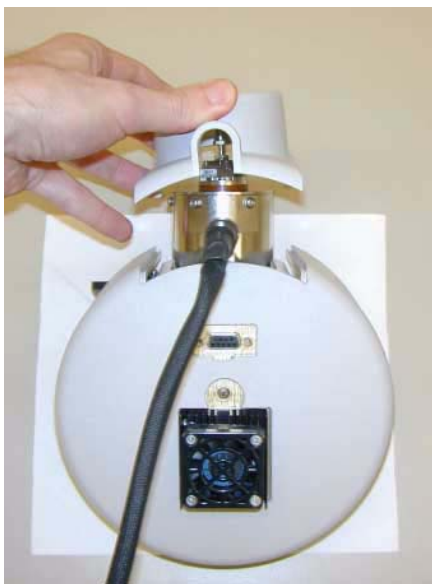
Figure 32 Removing the Nebulizer Cover (left) and Removing the Cosmetic Cover screws
