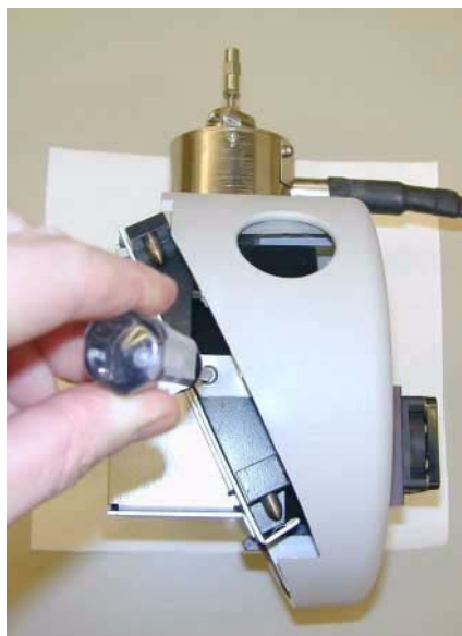
Figure 32 Removing the Nebulizer Cover (left) and Removing the Cosmetic Cover screws
