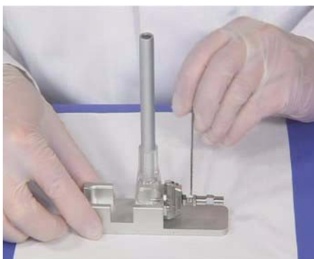
Figure 26 Installing the nebulizer in the adjustment fixture
