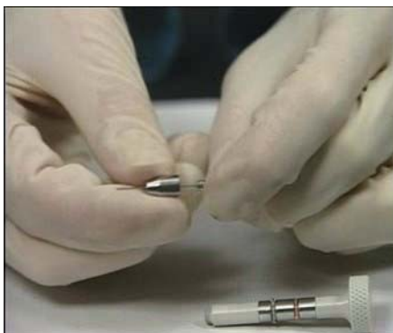
Figure 31 Installing a new needle into the collar
