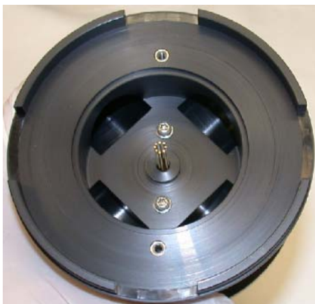
Figure 56 Octopole rods extending through Skimmer Spacer.
