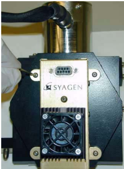
Figure 34 Use a 2 mm Hex Key (left) and Nylon Insulators
