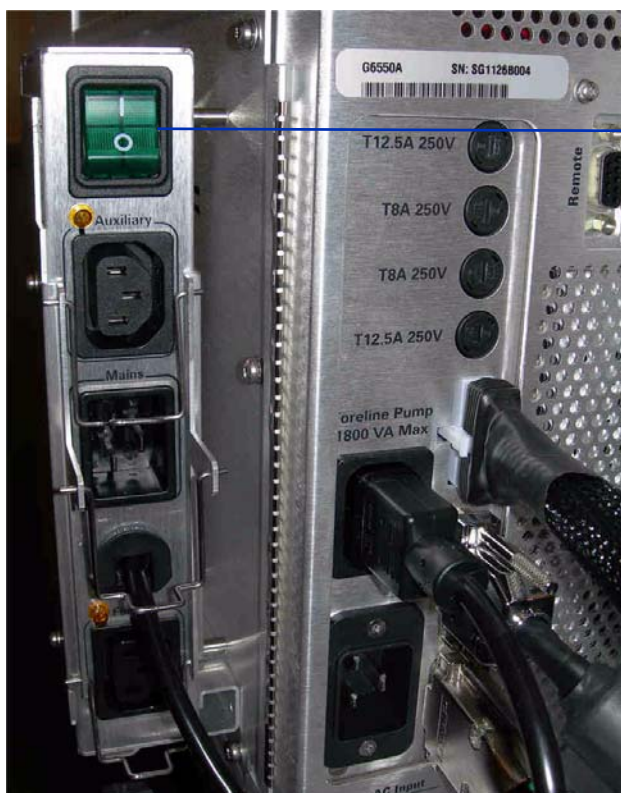
Figure 6 6550 power connections and pump expander box behind service panel
