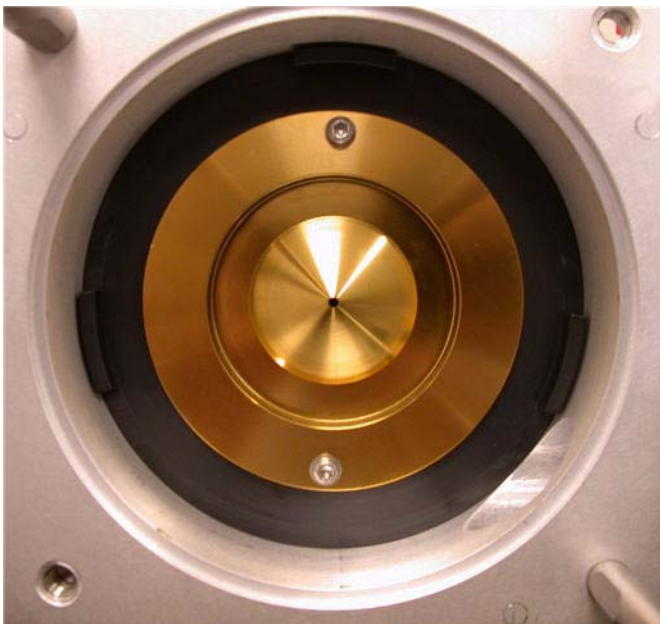
Figure 58 Example of a clean skimmer.
