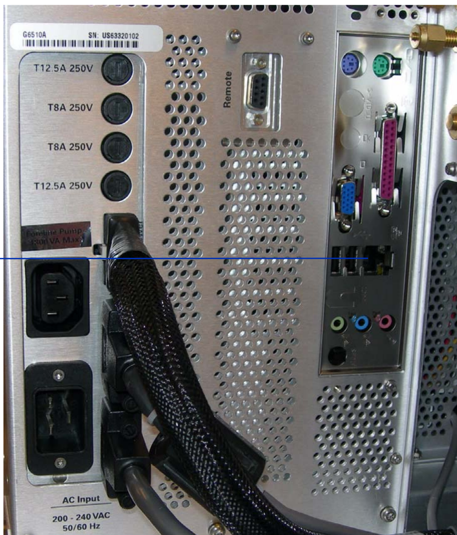
Figure 5 6520/6530/6538/6540 gas, LAN, and power connections behind service panel
